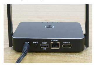
Step2. Keep pressing the "RESET" button with pen, paper clip, SIM ejector, etc. Then press "POWER" button to activate QuattroPod Receiver.
